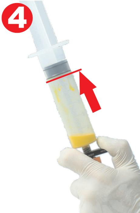
4. Pull the plunger of the syringe up to the maximum to create a vacuum within the cartridge. Now you see air bubbles rise in the ink. Please remain in this position until you do not see any air bubbles rise.
