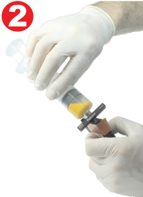
2. Prepare one of the included 60ml Luer-Lock syringes with the requested amount of ink. Redundant air should be removed as far as possible.
