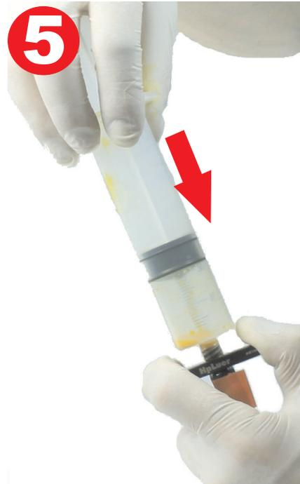
5. Release the plunger. The ink in the syringe will be soaked in by the vacuum. Meanwhile the plunger moves down. If the plunger stops moving, slightly press the remaining ink into the cartridge. The last step has to be a gentle pull movement to get a pressure compensation within the cartridge. Now remove the HPLuer. Please check the full weight.
